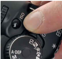
ABOVE Changing the ISO setting alters your DSLR sensor's sensitivity to light, also affecting the 'signal to noise' ratio. The higher the ISO, the more noise.
